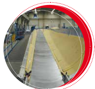
9 Further processing at the customer Laying into the mould
